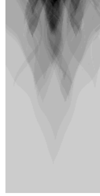
Figure 2. The numbers of travel times corresponding to the point source at the bottom of the model box, 1.55 km from the left-hand corner. The maximum number of travel times is 49.
